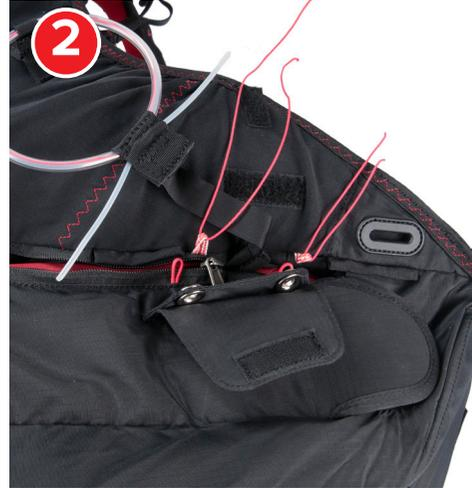
Make sure all lines are neatly on the bottom of the container, move zipper to the shown position and pass the paracord through the closing loops
