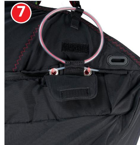
Remove the paracord slowly, place the handle flap on the velcro as shown
