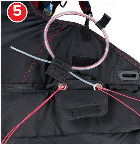
Pass the handle wires through the closure loops
