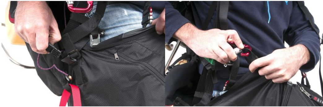
4 - Connect the lower right buckle of the cocoon to the harness and connect the right strap to the carabiner of your harness.
