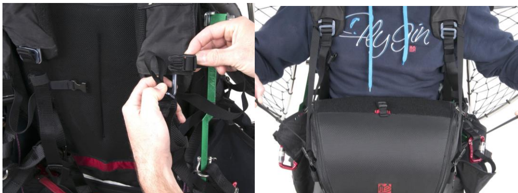
5 - If you use a lot of ballast, you can connect the cockpit to your shoulder straps. It will help support the weight during take off and landing. To do so, connect the straps to the buckles of the shoulder straps and adjust the length. Ballast
