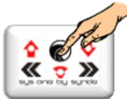
Press middle button for 2 seconds to turn ON and OFF the instrument.
